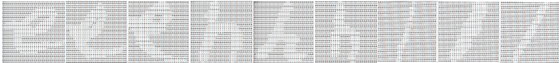
Fig. 2. Examples of some 32 \times 32 binary matrices that are used as input of the feature extraction phase. These examples correspond to characters e (left), h (center), and l (right).
